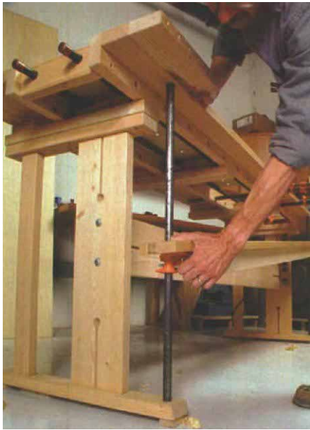
Sliding height adjustment. Pipe-clamp tailpieces slide on cast-iron pipes held captive in the top and bottom of the bench. A T-shaped Douglas fir planing beam rides on the clamps.
