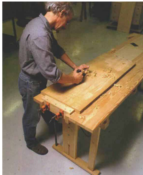
Horizontal clamps run full length. A pair of pipe clamps, running under the benchtop, hold work in the same way as a traditional tail vise.
