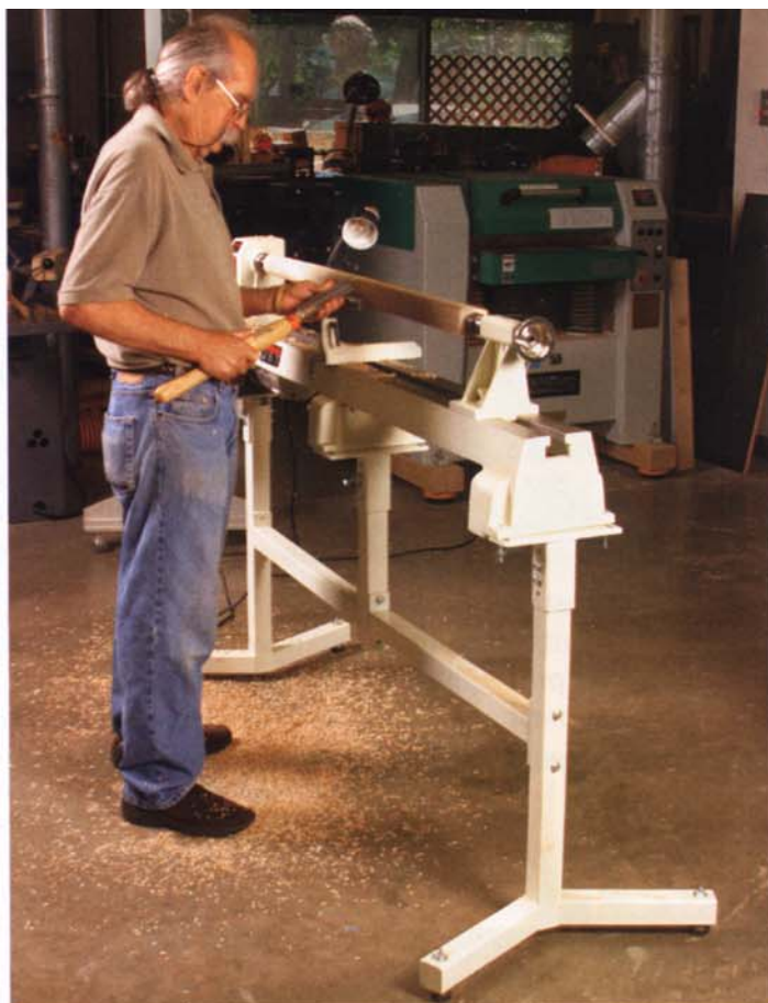
Accessories add capacity. An optional bed extension allows longer turnings, while a sturdy stand is height-adjustable.
