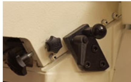
The handwheels (left) on both the infeed and outfeed tables make adjustments fast and easy. An easy-to-read scale is provided on the infeed side. This lockout (right) on the rear of infeed table prevents taking excessively deep cuts by accident. It limits cuts to 1/8" unless the operator disengages this limiter. It is easy to do but forces you to make a conscious decision to make very deep cuts.
