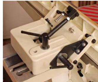
All of the fence controls and adjustments are grouped near the center for easy access.
