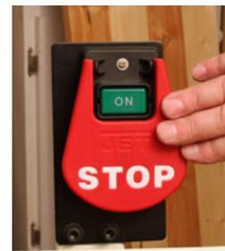
This paddles-style switch is mounted on a stalk on the JJ-6HHDX version. This puts the switch in easy reach and allows "bumping" the machine off.
