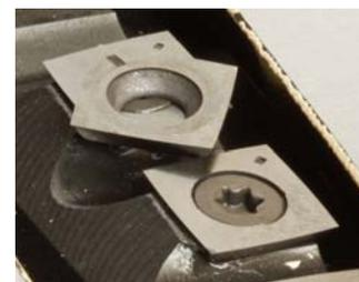
The helical head in the JJ-6HHDX version uses true carbide cutters, each with four identical cutting edges. Should an edge become dull or damaged, you can often turn it to a fresh edge (wrenches included) or replace it with one of the spare cutters included with the machine.
