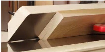
The large, cast iron fence tilts to 45-degrees in or out to handle all of your bevel work. It has adjustable stops at 90-degrees and both 45-degree settings.
