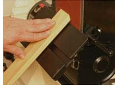
With the belt in the upright mode, the table can be tilted up to 45-degrees for precise trimming or forming. The miter gauge fits both the cast iron disc and this aluminum belt table.
