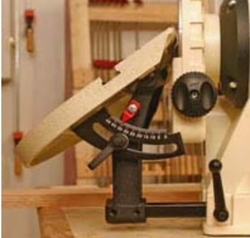
The cast iron table mounts on a single rod that can also be installed at the belt section. The table tilts to 45-degrees and features a handy scale.
