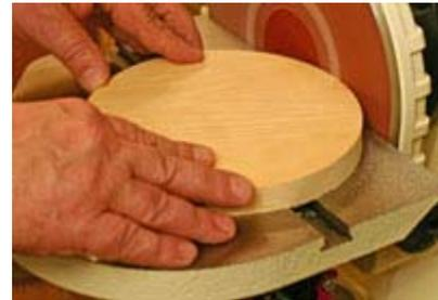
The specially designed center point (left) fits the miter slot on the cast iron table and makes sanding perfectly round disks (right) simple and very safe.
