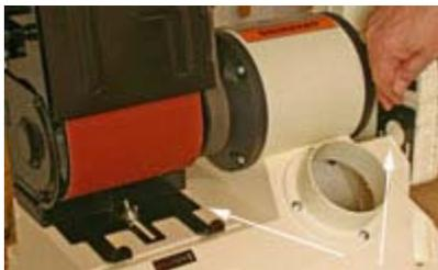
In addition to the 4"-diameter dust port, we included dust gates at the disc and belt section to maximize the suction where you need it.
