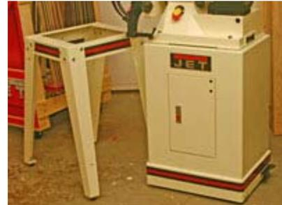
The JET JSG-96 is designed as a bench tool and has handholds designed into the case. However, we offer both closed and open stands to make it a stand-alone tool for easier more versatile access, particularly for large jobs.
