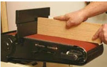
The belt can be positioned flat, as it is here or fully vertical.
